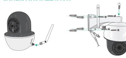
Screw the Antenna clockwise into the rear of the camera.
