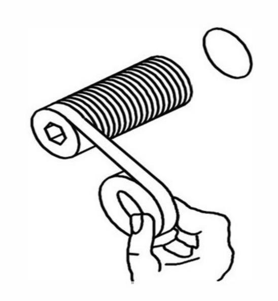
1.Wrap the sealing tape on the 1/2 NPT thread joint and connect the water pipe
