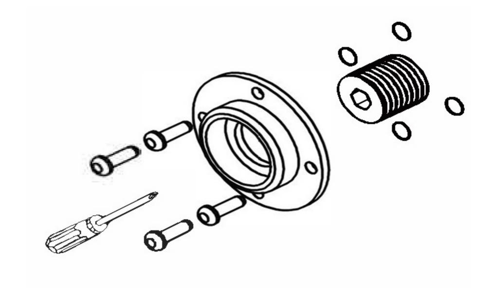
4. Fixing the base with screws
