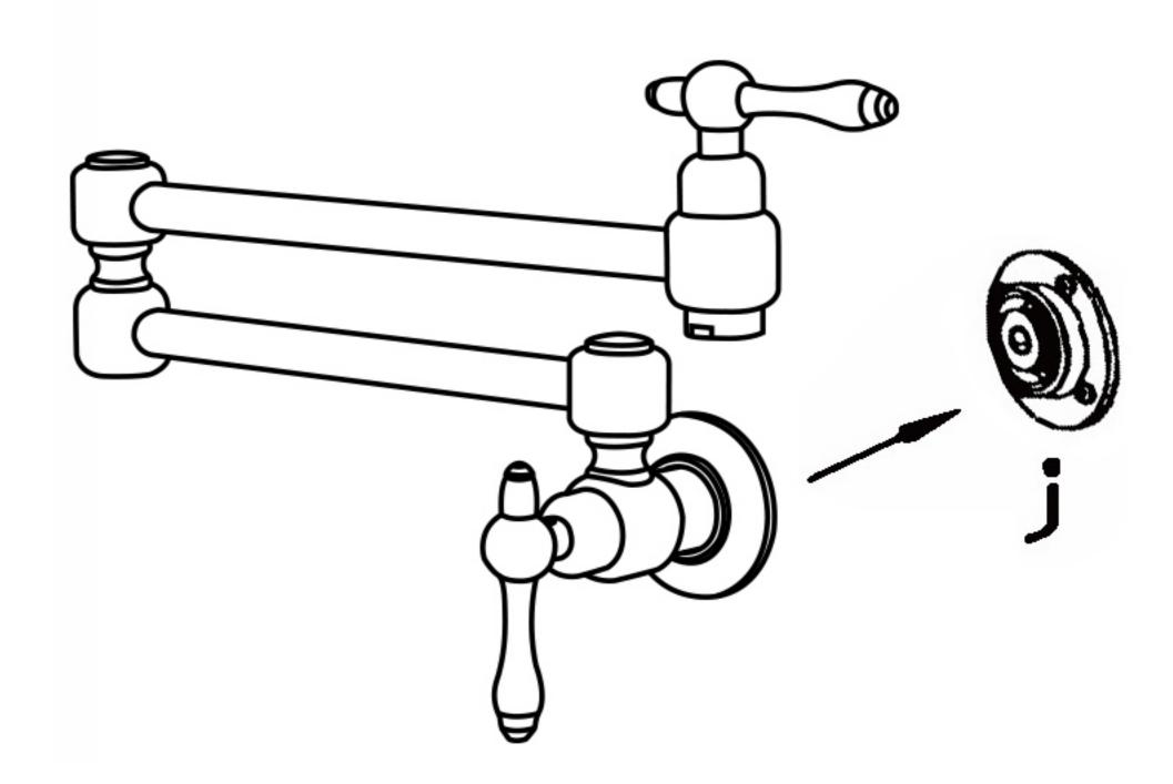
6.Connect the faucet to the thread joint on the wall, and use a hex wrench to tighten the screw from the side of the base to fix the base.
