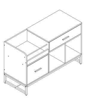
Notes:Don't tighten screws completely at first, just in case parts were assembled wrong and need disassembled. Tighten screws at last when all parts are put together.
