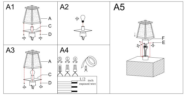
Step A1 » Unscrew knob nuts (D) from iron plate (C) and body (A), then set them aside for later installation.
