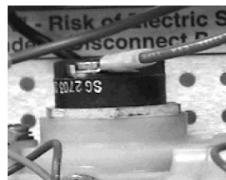
Figure 11: Installed heating element
