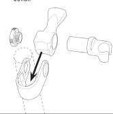
Screw Threaded Cap onto end of 6 Hand Shower Holder. A coin may be used to assist in tightening Cap; however, be careful not to over tighten.
