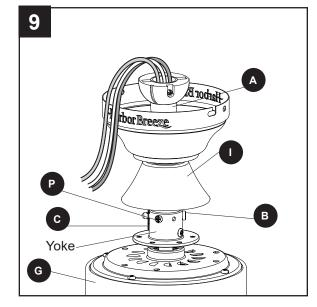
10. Depending on the length of downrod you use, you may need to cut the lead wires back to simplify the wiring. If you decide to cut back the lead wires, pull them all the way through the top of the downrod. Then measure 8 inches of lead wire and cut the excess wire off with wire cutters (not included).
