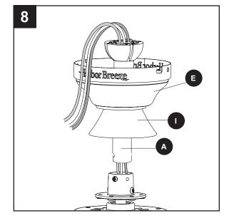
Slide the downrod (A) into the yoke of the motor assembly (G), align the holes, then re-install the downrod pin (B) and downrod clip (C). Secure with set screws (P) and slide the yoke cover (I) down until it rests on top of the motor assembly (G).
