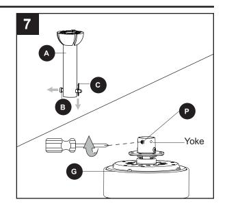
Insert the downrod (A) through the canopy (E) and yoke cover (I). Feed the wires from the fan through the downrod (A).
