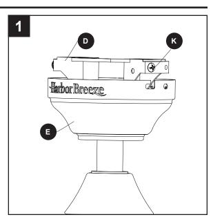
Secure the canopy (E) with the mounting bracket screws (K) previously removed (Step 4, page 8). Tighten all mounting bracket screws (K) securely.
