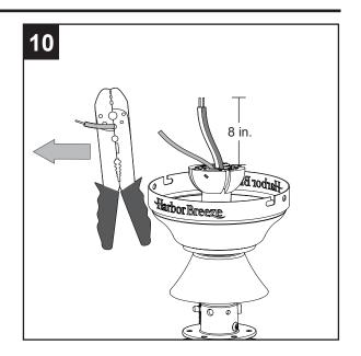
If you decided to cut back the lead wire in Step 10, strip 1/2 in. of insulation from the end of each wire. Twist the stripped ends of each strand of wire within the insulation with pliers (not included).
