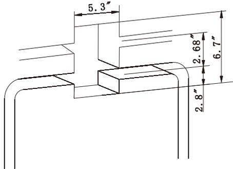
2. The depth of the embedded box is 1.8"-2.2". It's better to drill the depth of 1.8" for blank wall.
