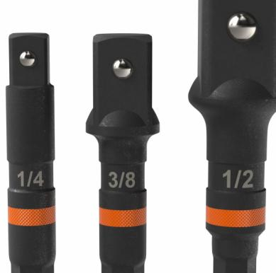
Klein Tools 3-Inch Impact Socket Adapter Set includes 1/4, 3/8, and 1/2-Inch square drive sizes for quick conversion from impact drivers to sockets. The knurled grip provides steady handling, even with oily or gloved hands, while the high-visibility orange band makes it easy to spot in a tool bag or dimly lit jobsites.
