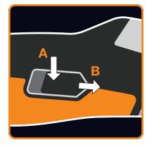
2. Press lock button (A) and slide until handle springs open (B).
