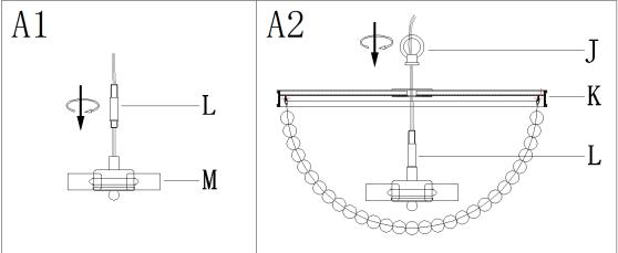
Step A1: Pass the fixture wires through the stem (L) and screw stem (L) onto the fixture loop assembly (M). Step A2: Pass stem (L) through ring (K) and secure with loop (J).
