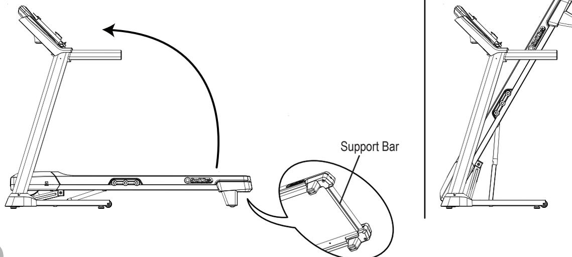
7. Make sure that the locking mechanism is engaged. Carefully pull back on the Walking Deck and make sure that it does not move. When you do this, keep clear of movement path in case the treadmill lock is not engaged.
