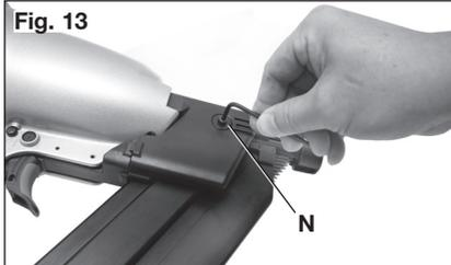
5. If nail still can not be removed, remove the magazine:
