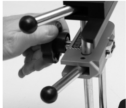
Step 7 - Turn the knob counterclockwise to return the blade to scoring position.
