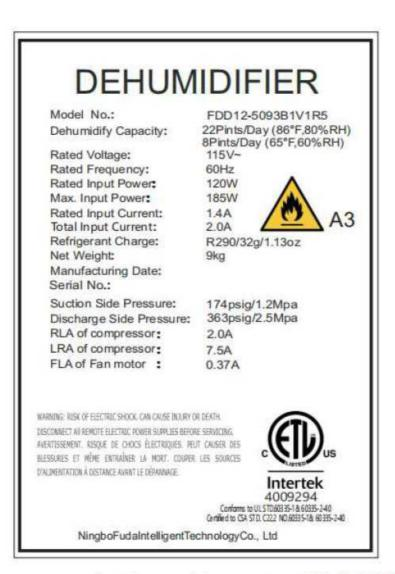
Remark: The parameters for other models are same as FDD12-5093B1V1R5, only model number on nameplate is different.
