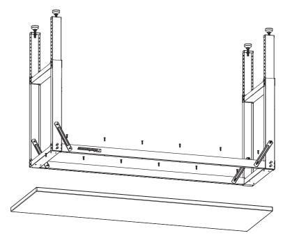
Turn the workbench upright and place in the location it will be used. Check to make sure the frame is still level. If you need to adjust, use the leveling feet.
