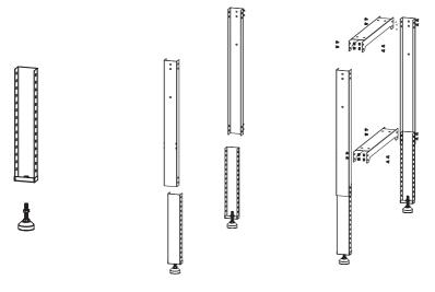
Take two of the four cross bar pieces and slip them together with the top flanges facing in opposite directions. (See figure at the bottom of page 7.) You will see three sets of four holes – you can join the two cross bars together at any of these hole patterns. (The other end of each cross bar only has two holes, which will attach to a leg assembly.)
