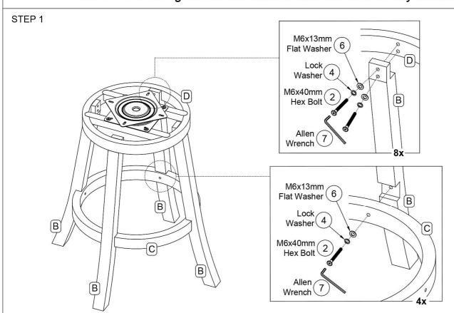
Attach the Chair Legs(Part B) to the Apron with Swivel Plate (Part D), then attach the Footrest (Part C) to inside of the Chair Legs(Part B) using (12) M6x40mm Hex Bolts (Part 2), (12) Lock Washers (Part 4), (12) M6x13mm Flat Washers (Part 6). Loosely tighten using Allen Wrench (Part 7).
