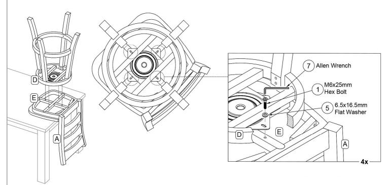
Keep the Backrest (Part A) and Wooden Seat (Part E) inverted on a stable raised surface. Attach the Swivel Plate located on the Apron with Swivel Plate (Part D) to the Wooden Seat (Part E) using (4) M6x25mm Hex Bolts (Part 1) and (4) 6.5x16.5mm Flat Washers (Part 5) Tighten all screws using Allen Wrench (Part 7). Return Chair to the upright position.
