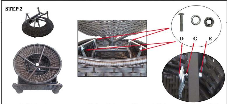
One end of Swing Arms are pre-assembled on Chair Base (C). Attach Chair Base (C) to assembled Chair Bucket (A) and Chair Skirt (B) and secure the other end of Swing Arms to two steel bars on Chair Skirt (B) with 4pcs Long Bolts (D), 4pcs Washers (G) and Nuts (E) by using Allen Wrench (I) and Wrench (J) as shown in diagrams above.
