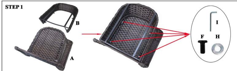
Lie Chair Bucket (A) upside down on the gournd. Assemble Chair Skirt (B) to Chair Bucket (A) with Short Bolt (F) and Flat Washer (H) by using Allen Wrench (I) as shown in a diagram above.
