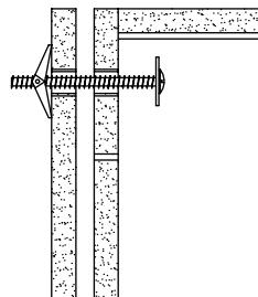
**DRY WALL** Drill holes and secure to the wall with toggle bolts and a washer.
