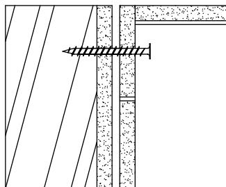
**STUD WALL** Secure to wall with #12 x 2" screws with a washer at stud locations.
