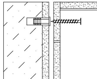
**CONCRETE WALL** Drill 1/4" holes, insert #12 wall anchors and secure to wall with #12 x 2" screws.
