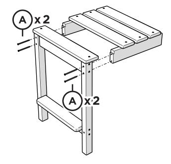
Pre-drilled holes indicate screw placement only. Fully thread screws into material for full engagement
