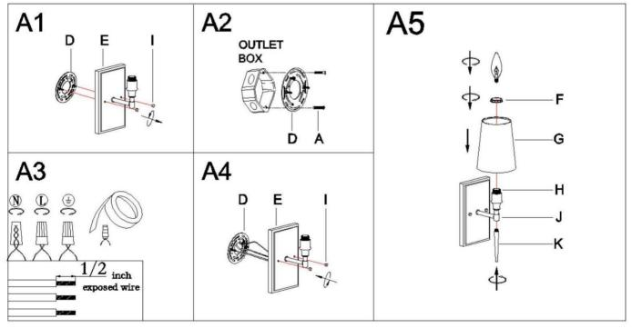
Step A1: Unscrew the ball knobs (I) from the back plate(E) then gently remove the mounting plate (D). Step A2: Secure mounting plate (D) to outlet box with mounting screws (A).
