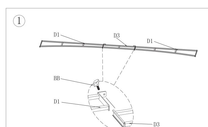
Please find 2 PCS of D1 and assemble them into each end of D3 by using Screws BB.
