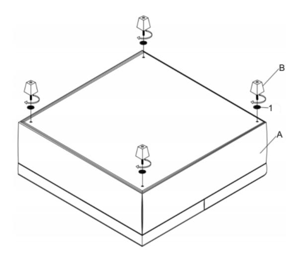
Place the Ottoman (A) on its back on a flat smooth surface. Attach the Feet (B) with Washer (1) to each corner.
