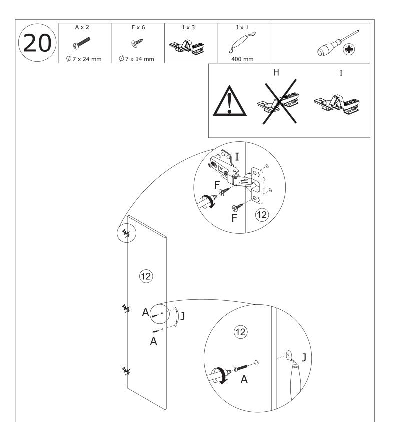
Fix hinge(I) to another plate 12 using screw(F) as shown. Fix handle(J) using screw(A) as shown.
