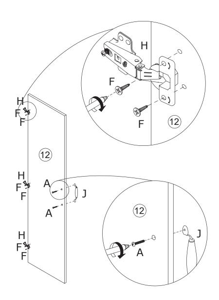
Fix hinge(H) to plate 12(x2) using screw(F) as shown. Fix handle(J) using screw(A) as shown.
