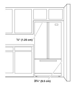
To ensure proper ventilation for your refrigerator, allow for a  $\frac{1}{2}$ " (1.25 cm) of space on each side and at the top. Allow for a 1" (2.54 cm) space behind the refrigerator. If your refrigerator has an ice maker, allow extra space at the back for the water line connections. When installing your refrigerator next to a fixed wall, leave a 3%" (9.5 cm) minimum space between the refrigerator and wall to allow the door to swing open.
