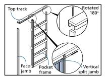
5. Set pocket frame and face jamb into the rough opening. Shim 4" from the corners and at 24" maximum intervals until square, level, and plumb.
