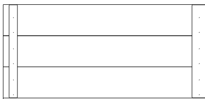
RP5 | RIGHT PORCH ROOF PANEL - W2A02629 (1) 1 5/8"x15 5/8"x32 7/8" (42x396x834)
