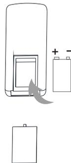
Install with a suitable battery
