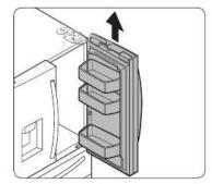
4. Open the door 90 degrees. While holding the door, pull up and remove the top hinge. Be careful not to damage the connector wires when you remove the hinge.
