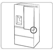
Check the height difference between the doors, and then lift up and hold the door with the lower height.
