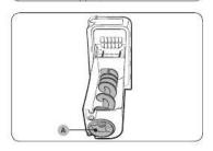
If the ice bucket is not firmly inserted, turn the **Helix (A)** 90 degrees, and then try again.
