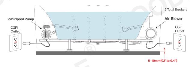
For Air Bath and Whirpool Tub installation, Do not apply any silicone sealant after installation, leave a 5-10mm(0.2" to 0.4")gap for motor/pump ventilation purpose.
