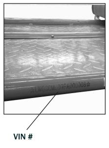
The Vehicle identification number is needed when calling for parts, service center help or when registering your Go Kart. Locate the number and list the number below for your reference.
