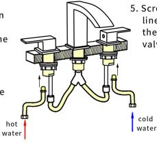
5. Screw the water supply lines to the faucet body,the handles and the stop valves
