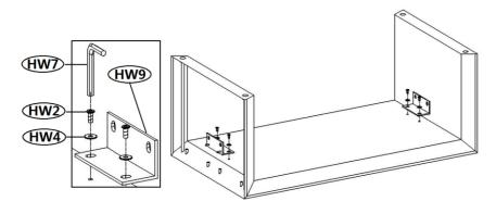
Step 3: Align the Steel corner(HW9) to the holes on Table top and Leg board, put the Flat washer(HW4) on the Hex bolt(HW2), insert it into the hole, tighten them by using Allen key(HW7).
