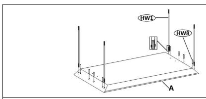
Step 1: Insert the Lead screw(HW1) and Wooden dowel(HW8) into the holes on Table Top(A) in order.
