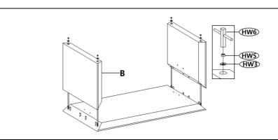
Step 2: Cross the Lead screws, put the Leg board(B) on the Table top. Put the Flat washer(HW3) and Nut(HW5) on lead screw, tighten them by using Socket wrench(HW6).
