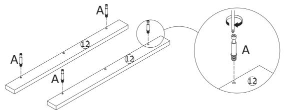
Insert quickfit screw(A) into corresponding holes in two plate 12 with screwdriver as shown.
