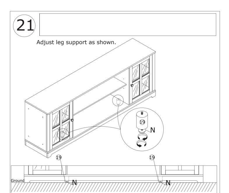
If the cabinet is unstable with the ground, please rotate the 19 # foot fitting (N)
