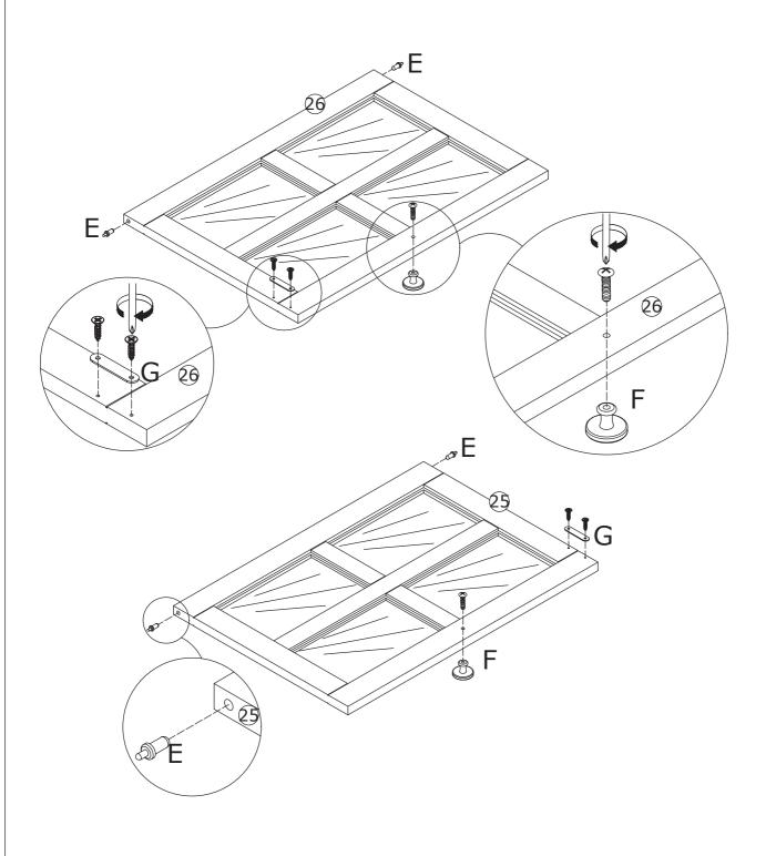
Assembled the two door plate as shown.
