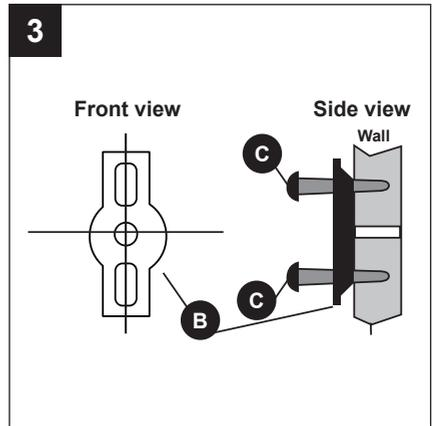
4. If attaching into drywall without a wood stud, drill 1/4" holes in the drywall through the mounting screw holes in each mounting bracket (B). Gently hammer the drywall anchors (A) into the holes until flush with the wall surface. Fasten the mounting brackets (B) to the wall with mounting screws (C).
