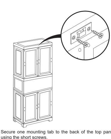
Secure one mounting tab to the back of the top panel using the short screws.
