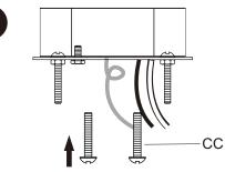
□ Install the lamp onto the hanging board
