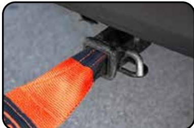
2. Attach the other end of the strap to the vehicle you are using to pull with. Many vehicles have hooks or loops you can use to do this. You can also use a trailer hitch receiver with a bolt/pin as shown.
