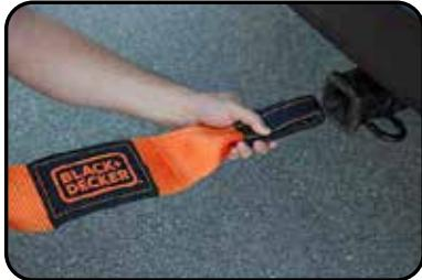
1. Connect the recovery strap to the machine / vehicle that is disabled / stuck by threading the end of the recovery strap through the vehicle's tow hook. Some vehicles have a hidden hook location behind a small square piece of plastic that is removable.
