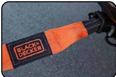
3. Once the strap is attached to both vehicles, drive very slowly to take out the extra slack in the strap. Once the strap is taut, slowly accelerate at very low speed until the disabled vehicle is free. Sudden tugs may lead to damage to either of the vehicles or the strap.
