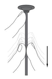
The length of the cable is adjustable. To determine the proper length of the fixture, hold the fixture canopy up against the outlet box in the ceiling to adjust the cable.
