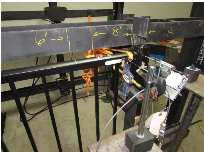
Typical Concentrated Load at Post Test Setup
