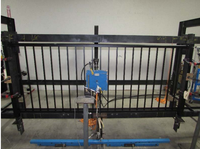
Typical Infill Load Test Setup (Near Center of Balusters)
