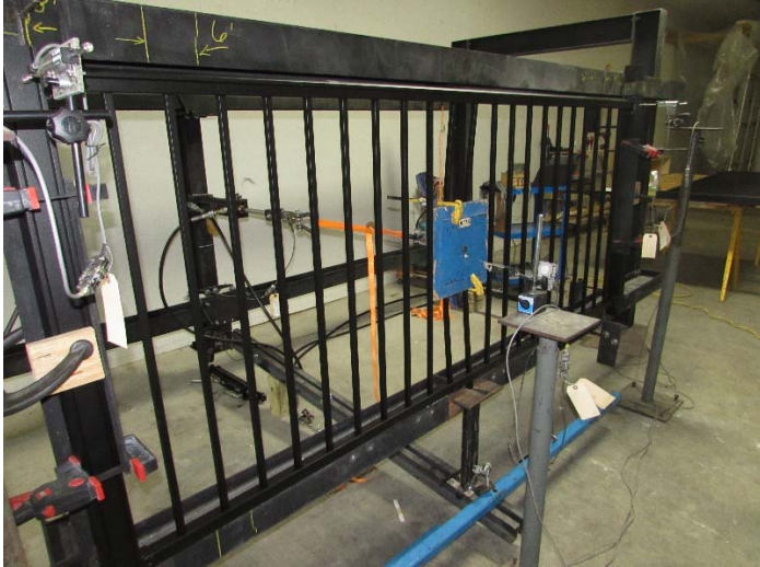
Typical Infill Load (Center) w/ Full Load Applied
