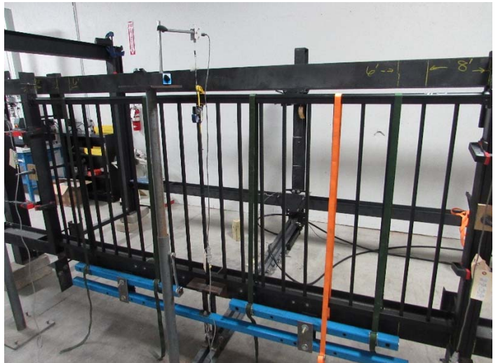
Typical Vertical Uniform Load Test Setup
