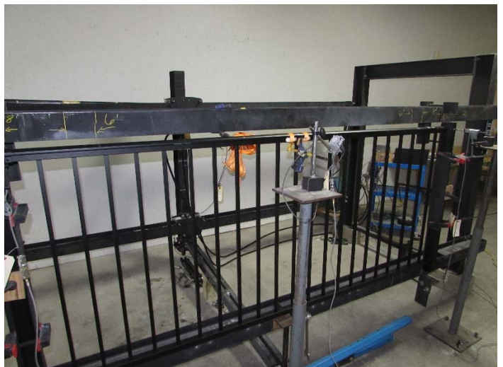
Typical Concentrated Load at Midspan Test Setup
