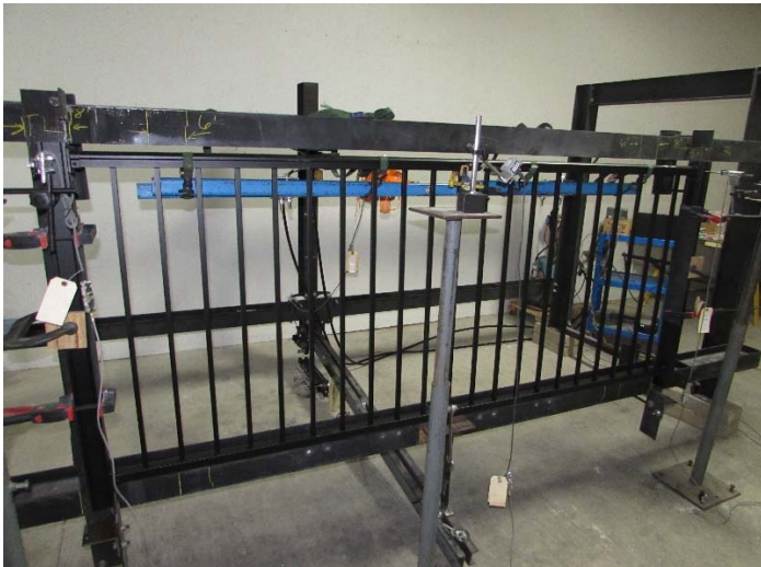
Typical Horizontal Uniform Load Test Setup
