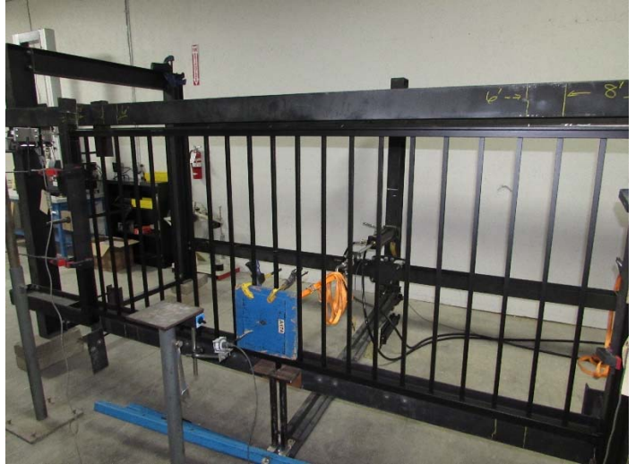
Typical Infill Load Test Setup (Near Bottom Rail)
