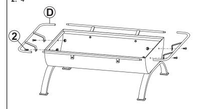
Align Curved Rails (D) with the straight rails and the short side of the fire bowl. Loosely secure the curved rails by hand-tightening four M6x12mm Bolt Sets (2).
