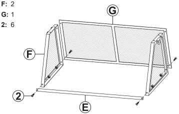
NOTE: The front of the side screen has one mounting hole, the back has two mounting holes.
