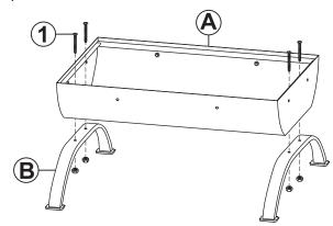
Align Fire Bowl (A) onto Legs (B) and secure using four M6x30mm Bolt Sets (1).
