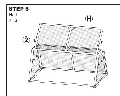
**IMPORTANT:** The top of the front screen installs on the inside of the side screens, while the front of the spark screen remains on the outside of the side screens.
