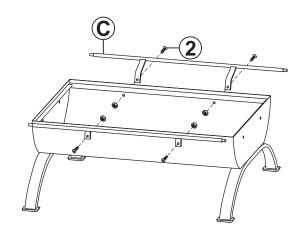
Align Straight Rails (C) with the long sides of the fire bowl and loosely secure by hand-tightening four M6x12mm Bolt Sets (2).
