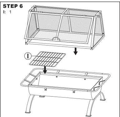
Place Cooking Grate (I) onto the ledges inside the fire bowl. Then, place the spark screen over the fire bowl.
