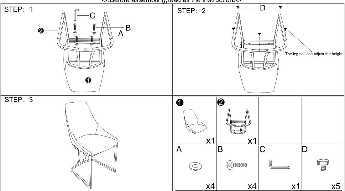
Note: Put all the screws into the hole site, And then tighten them. Do not tighten one by one
