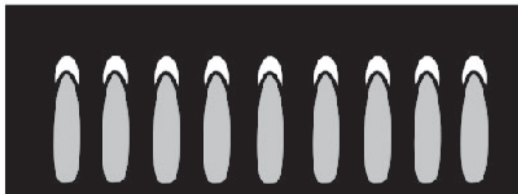
(B) Yellow tips on outer cones— Normal for propane gas
