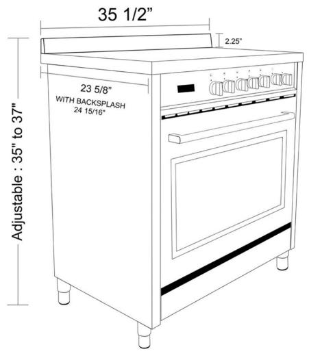
Overall Interior Oven Dimensions (WxDxH): 26.5" x 18" x 14" Usable Interior Oven Dimensions (WxDxH): 26.5" x 16.75" x 11.5"
