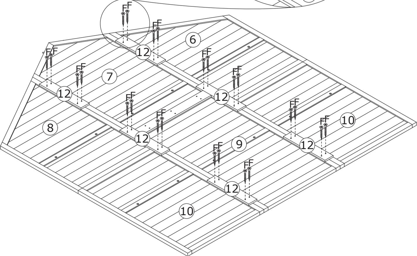
Fix plate 12 to plate 6, 7, 8, 9 and 10 with screw(F) as shown.
