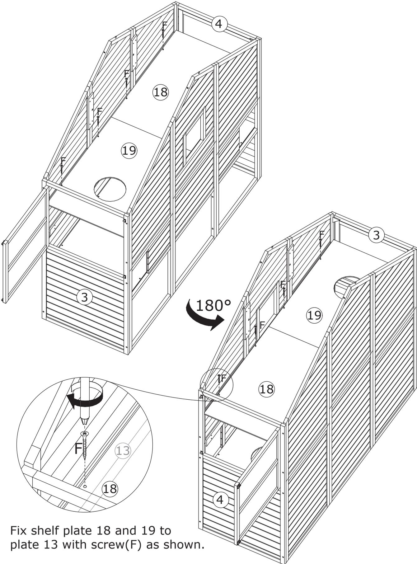
Fix shelf plate 18 and 19 to plate 13 with screw(F) as shown.
