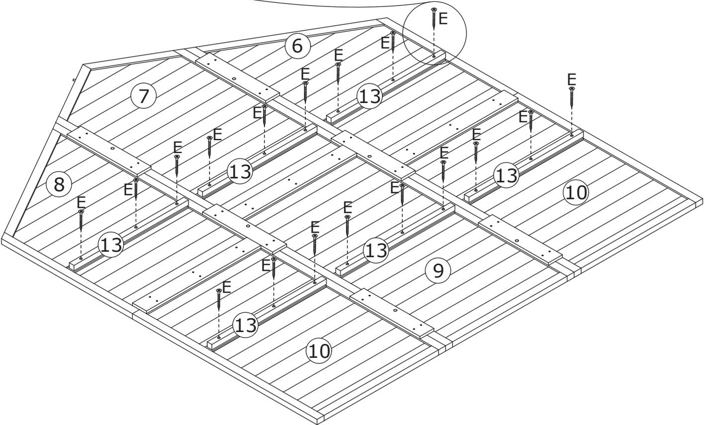
Fix plate 13 to plate 6, 7, 8, 9 and 10 with screw(E) as shown.
