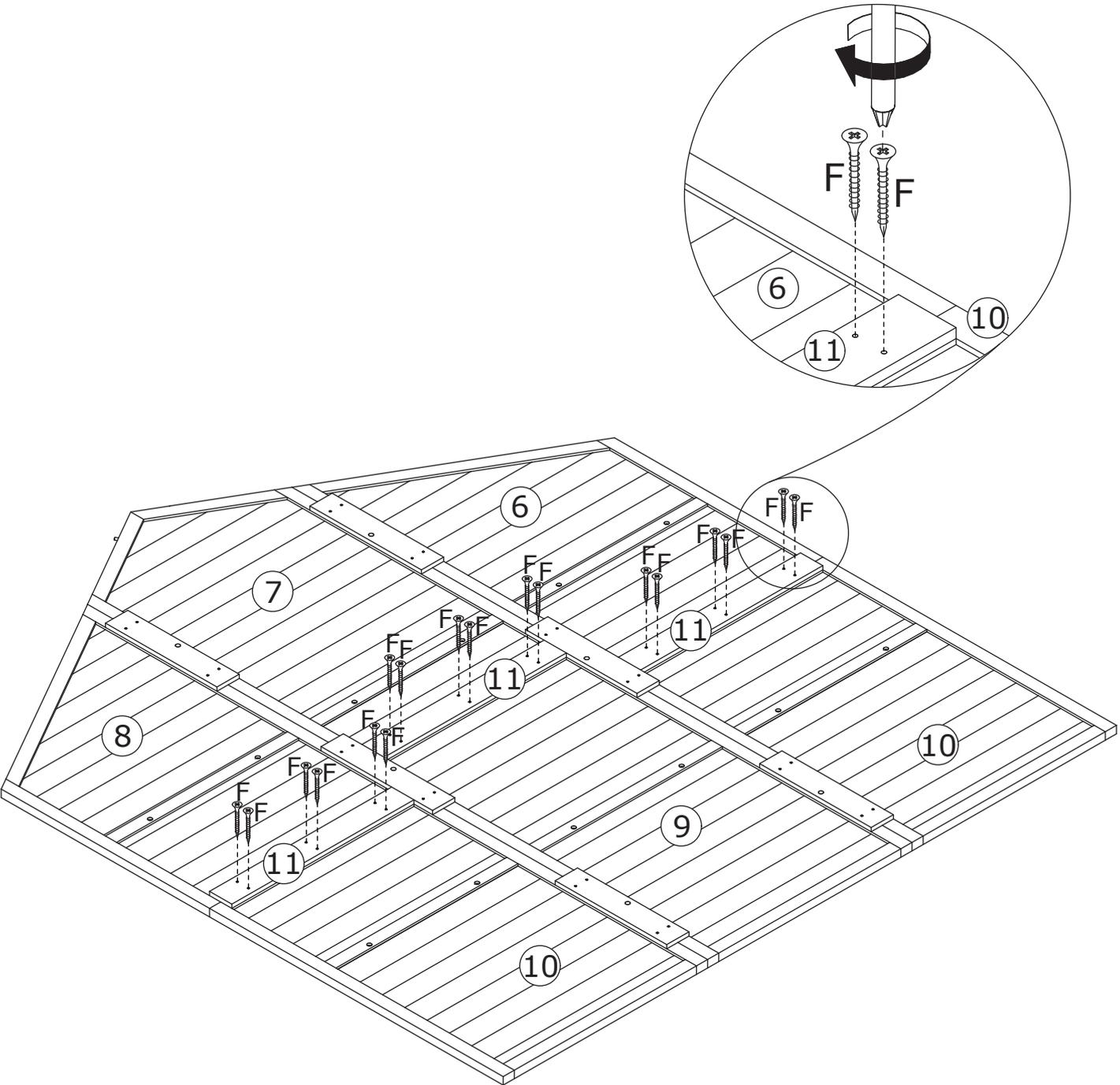
Fix plate 11 to plate 8 and 10 with screw(F) as shown.
