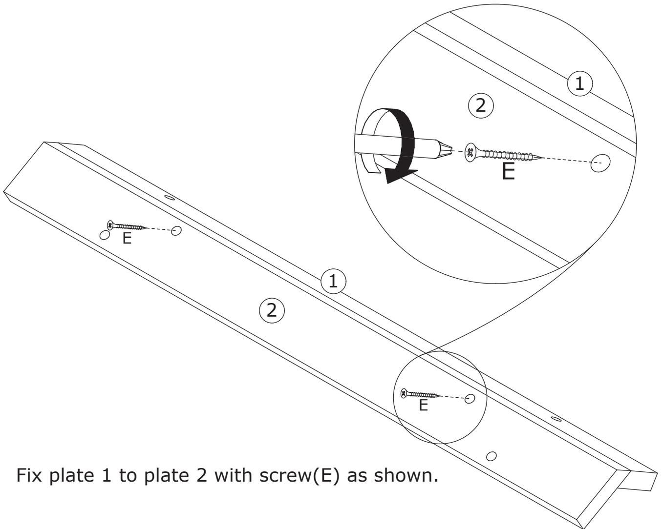
Fix plate 1 to plate 2 with screw(E) as shown.
