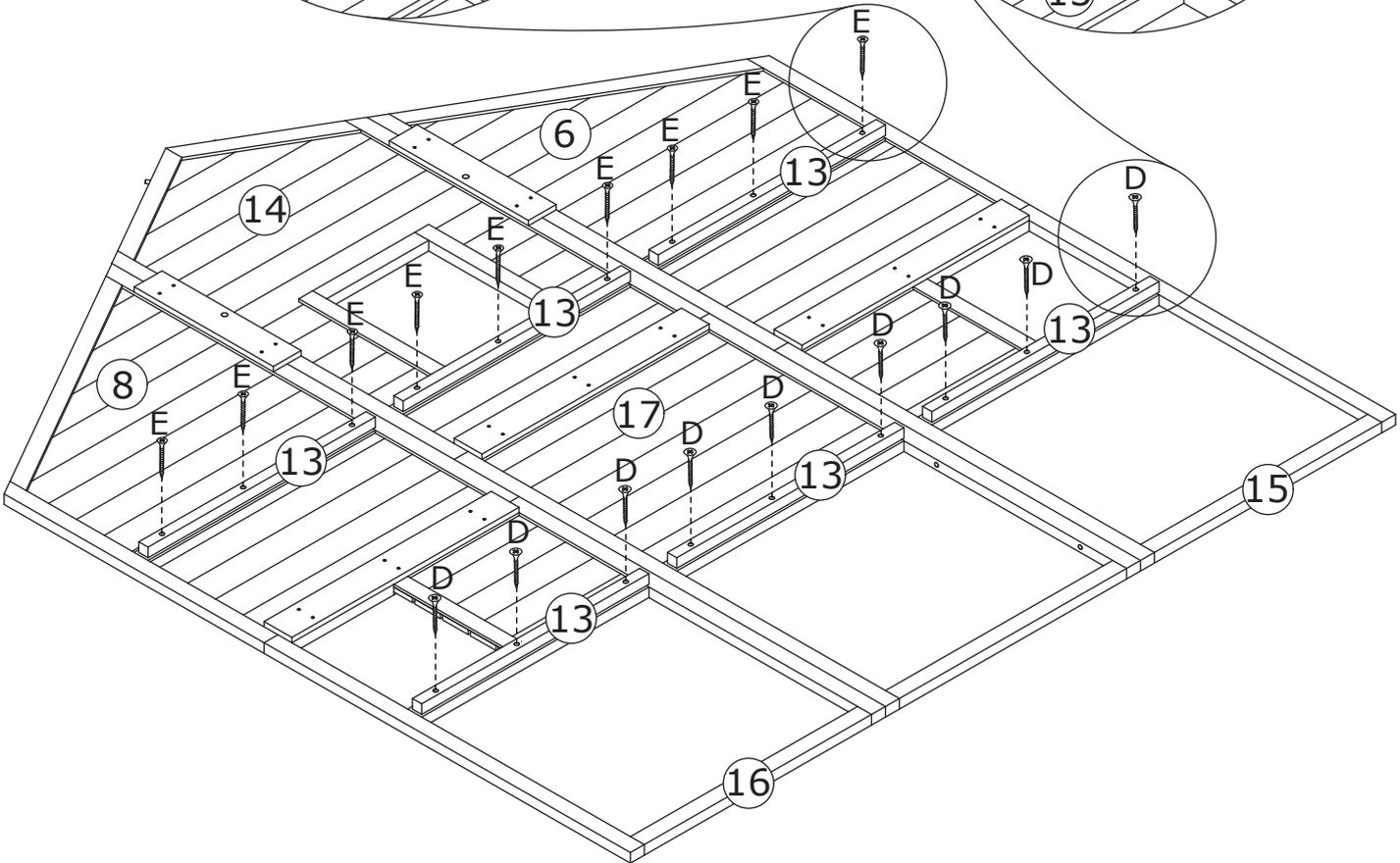
Fix plate 13 to plate 6, 8 and 14 with screw(E) as shown.
