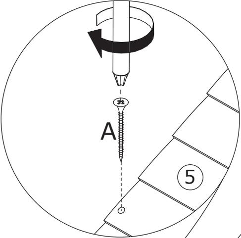
Fix top plate 5 to plate 6, 14, 7 and 8 with screw(A) as shown.
