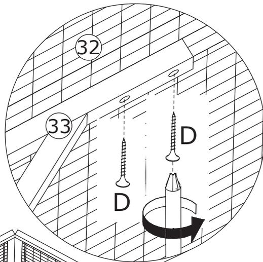
Fix plate 33 to plate 21, 22 and 32 with screw(D) as shown.
