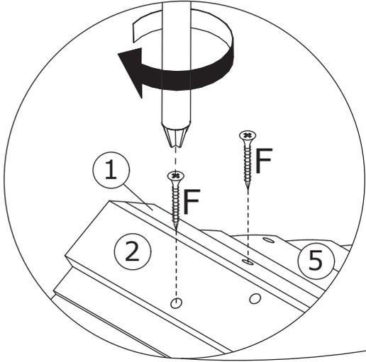
Fix plate 1 and 2 to plate 5 with screw(F) as shown.
