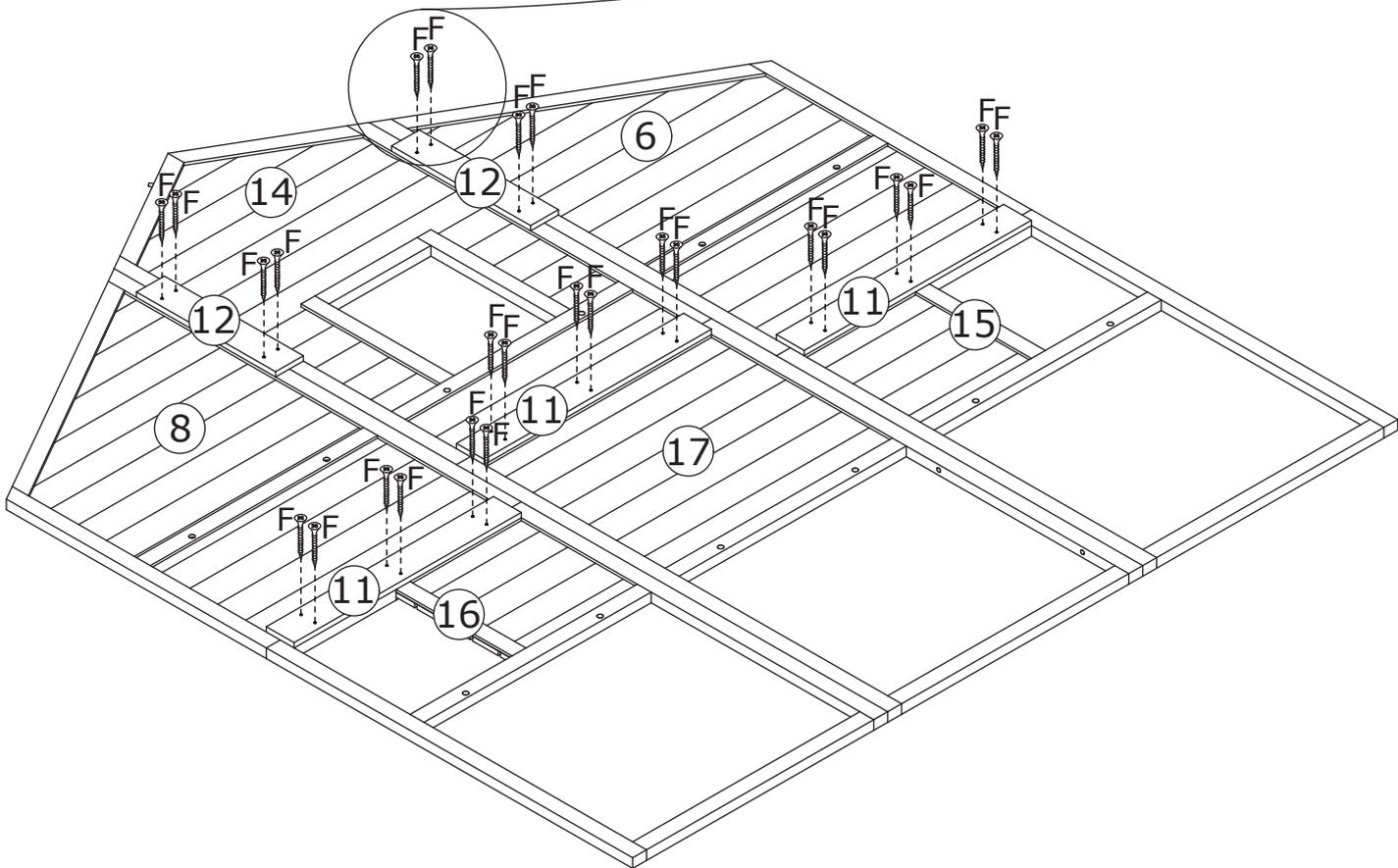
Fix plate 12 to plate 8, 6 and 14 with screw(F) as shown.
