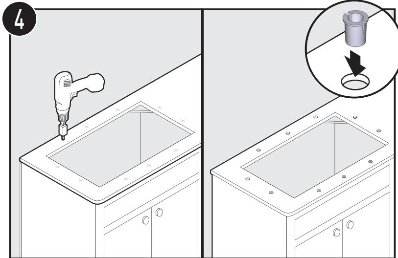
Drilling and anchoring may be required at this stage of installation. Locate and drill the mounting holes (following the countertop manufacturer's instructions) as shown. Holes should allow even spacing of mounting brackets around the sink. Type of fasteners to be as recommended by countertop supplier.
