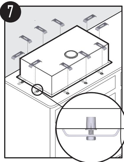
Attach mounting hardware. Consult your professional installer. Hardware can vary. Position brackets so that bracket edge overlaps sink ledge and finish installing mounting hardware.
