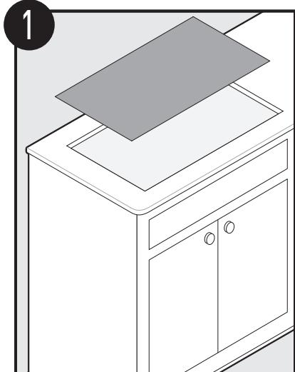
A fabricator can use the enclosed paper pattern to create the countertop holes for sink and/or faucet.
