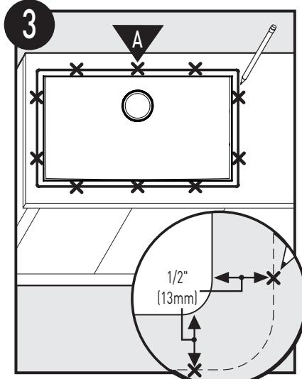
Determine location for mounting brackets; space evenly around the underside. Mounting holes should be 1/2" out from the edge of the sink ledge.
