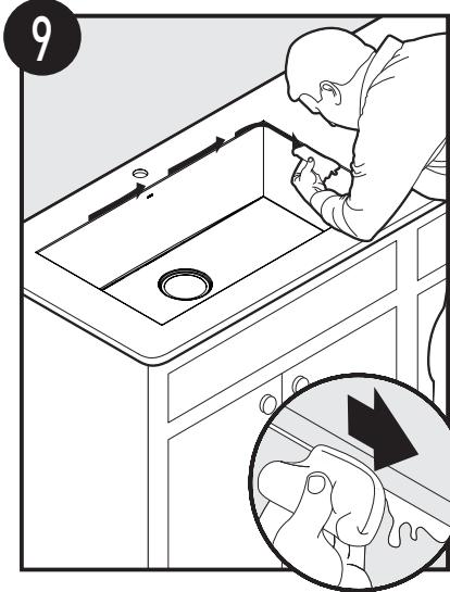
Complete counter installation and wipe away any excess caulk from sink rim.
