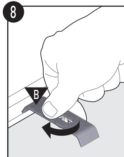
Tighten brackets evenly. Do not over-tighten. Turn countertop and sink attached right side up.
