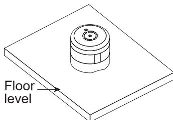
3. For floor or flat surface installation, re-connect the top (alarm) and base (sensor) and place it directly on the surface near the area to be monitored.
