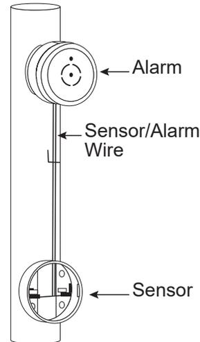
4. For installation in a sump pit, the alarm can be kept as an assembled unit (top and base together) and attached to the sump pump discharge pipe. Or, the base (sensor) can be separated and attached to the sump pump discharge pipe. The 5 ft. sensor-alarm wire allows the alarm to be mounted above the sump basin for easy accessibility.
