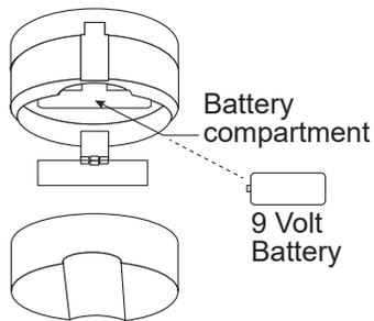
1. Separate the top (alarm) and base (sensor) of the unit to access the battery compartment.
