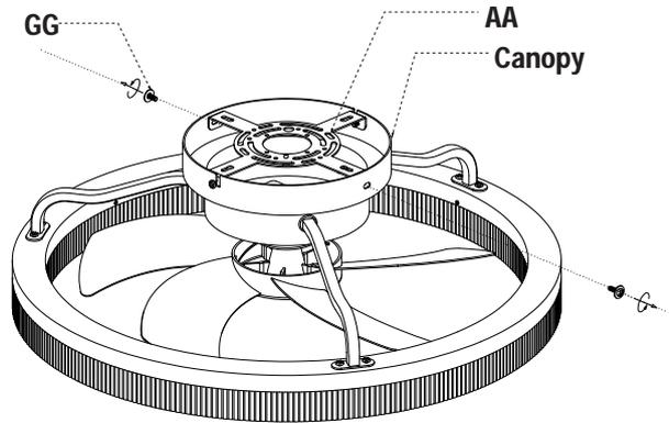
Step 1: Loosen and remove the canopy screws (GG) from the round holes, and loosen the canopy screws (GG) in the 'L' holes but do not remove them, and then remove the mounting bracket (AA) from the canopy.
