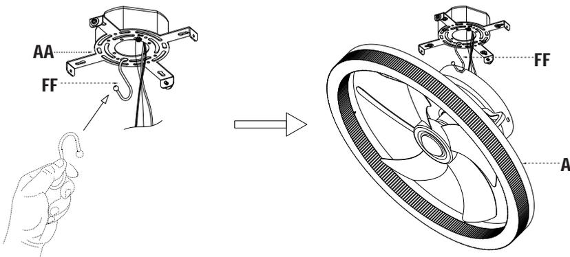
Hang the fixture onto the mounting bracket (AA) with "S" hook (FF) provided.
