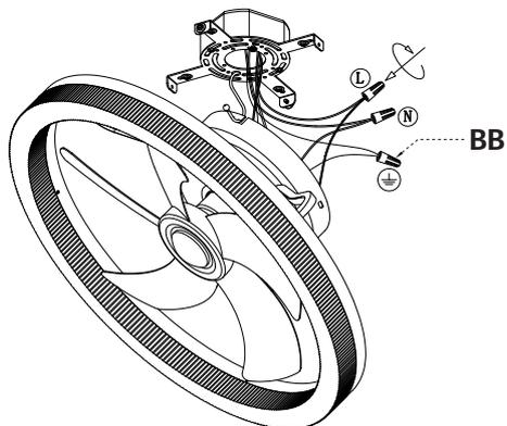
**Step 1:** Connect the wires from the fan to the house supply wires with wire nuts (BB), ground wire (green, green/yellow, or bare copper) to ground wire, neutral wire (white) to neutral wire, and hot wire (black) to hot wire. Wrap the connection with electrical tape.
