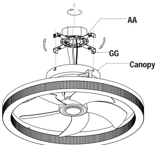
Align the "L" slots from the canopy to the canopy screws (GG) on the mounting bracket (AA), rotate the canopy to lock it onto the mounting bracket (AA).
