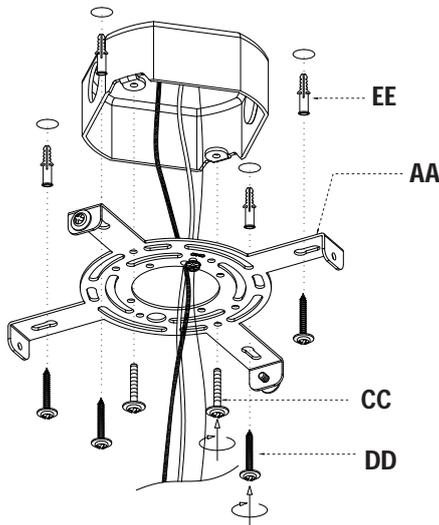
Step 2: Mark and drill screw holes in the ceiling, then insert the long plastic anchors (EE).
