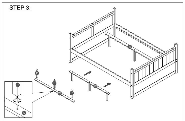
Assembling leg support (P) with lower support slat (W) later rotate, Move support slat inside Full bunkbed.
