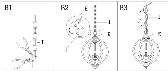
Step B1: By measuring, determine the correct number of links needed for proper hanging height. Using the chain pliers, disconnect and discard the remaining chain.
