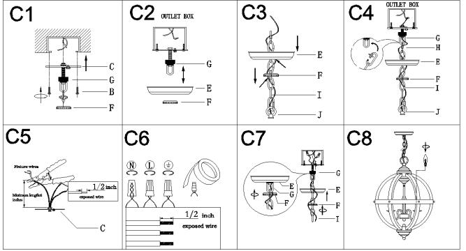
Step C1: Remove the threaded ring (F) from collar loop(G).
